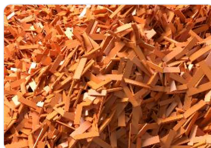
True polyhedra: lath shaped particles with a 1:25 aspect ratio in a twin screw feeder.
