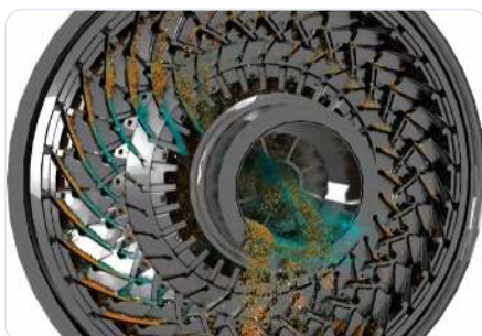
DEM coupled with SPH: ore and slurry through the pulp lifters of a full scale SAG mill.
