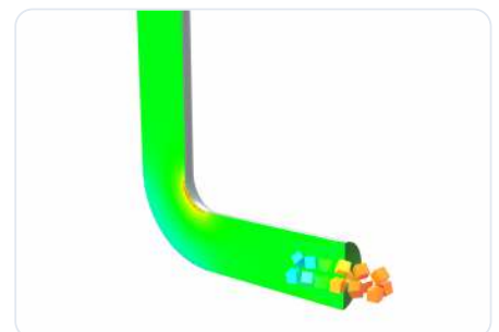
CFD - DEM: polyhedral particles carried through a pipe bend with OpenFOAM.
