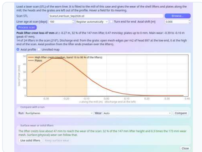
Wear scan: the scan fitted to the mill, with the loss of liner along the mill.
